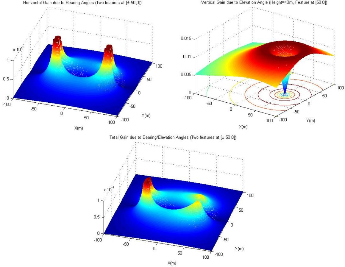
Figure 4: The information gain for the Case-1: (Top left) the horizontal information gain due to two bearing observations. (Top right) the vertical contribution from a single elevation observation. (Bottom) the combined total information gain. In this analysis, two landmarks are located at  $(\pm 50, 0, 0)$  and the vehicle has a constant height of 40m. Note the the zero-gain effect of the  $90^\circ$  elevation on the vertical information gain.
