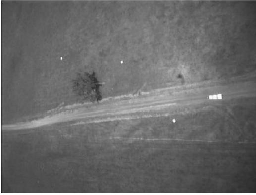
Figure 2: An example of aerial down-looking camera outputs. Features detected are represented in pixel coordinates  $(u, v)$  and are converted to bearing and elevation  $(\phi, \theta)$  to be fused in the navigation system.
