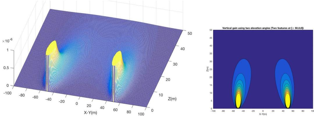
Figure 5: The height information gain for the Case-2 using two elevation angles; 3D plot (left) and 2D plot (right). The figures show the vertical section of the sensing geometry assuming the vehicle follows a straight line connecting two landmarks located at  $[\pm 50, 0]$ . It can be seen that the height information increases as the vehicle flies closer to the landmarks as well as maintaining the relative elevation angle as  $90^\circ$ .
