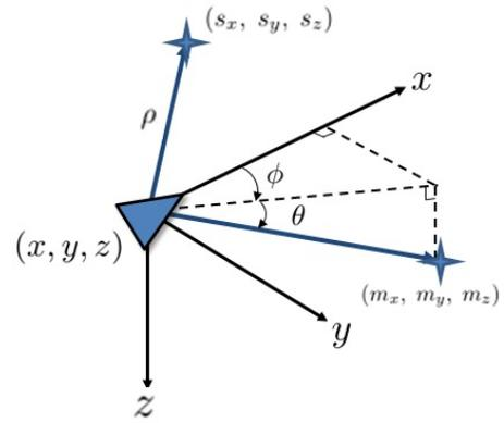
Figure 3: The sensing diagram for pseudorange ( $\rho$ ), bearing ( $\phi$ ) and elevation ( $\theta$ ) observations. All the satellite and landmark positions are expressed in a body-coordinate system:  $x$ (roll),  $y$ (pitch) and  $z$ (yaw).  $(s_x, s_y, s_z)$  and  $(m_x, m_y, m_z)$  are the satellite and landmark position, respectively.
