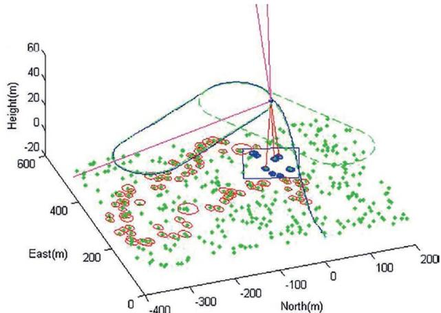
Figure 1: A sensing scenario used in this work showing GPS pseudoranges (3 skywards rays) and visual bearing/elevations (3 down-looking rays). The diagram shows an aerial SLAM simulation with with estimated landmark positions and uncertainties (blue - active map; red - inactive map; green - true map).
