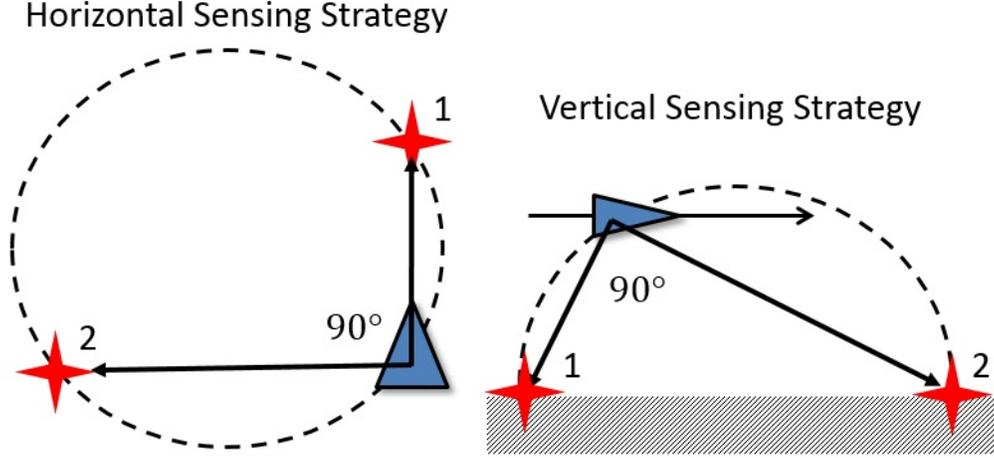
Figure 6: An optimal sensing strategy to improve the horizontal accuracy using two bearing observations (left) and an optimal strategy to improve the vertical accuracy using two elevation observations (right).
