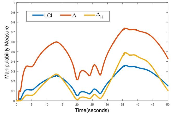
Figure 7: Graph of LCI,  $\Delta$  and  $\Delta_H$  manipulability measures during CRAM simulation
