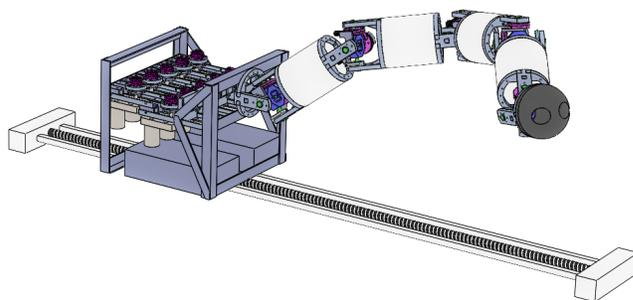
Figure 1: A 3D model of the proposed 12 DoF CRAM system, showing the translating base, 2 DoF joints and replaceable end effector
