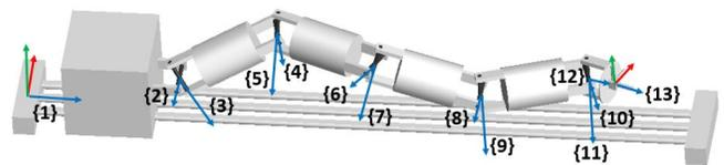
Figure 2: A simplified model of the 12-DoF CRAM system showing the setup of coordinate frames with  $x$ ,  $y$ , and  $z$ , where frame  $\{1\}$  is the base frame and  $\{13\}$  is the end effector frame
