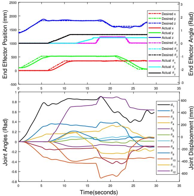
Figure 6: Graph of desired pose vs actual pose (top), with joint angles (bottom) showing effectiveness of self motion for joint angle reduction
