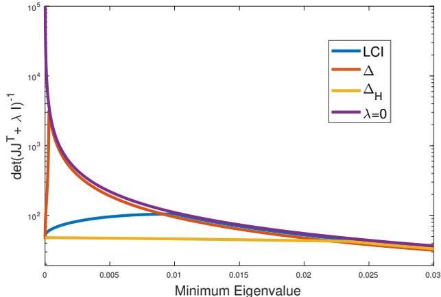
Figure 4: Graph of  $\det(JJ^T + \lambda I)^{-1}$  using LCI,  $\Delta$  and  $\Delta_H$  manipulability measures for damping, as a function of the minimum eigenvalue  $\omega_1$ , with  $\omega_2 = \omega_3 = 1$
