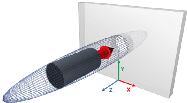
Figure 5: An example of the use of a task ellipsoid for an operation in which a peg has to be inserted into a hole
