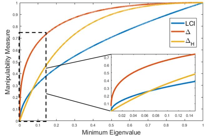
Figure 3: Graph of LCI,  $\Delta$  and  $\Delta_H$  manipulability measures as a function of the minimum eigenvalue  $\omega_1$ , with  $\omega_2 = \omega_3 = 1$
