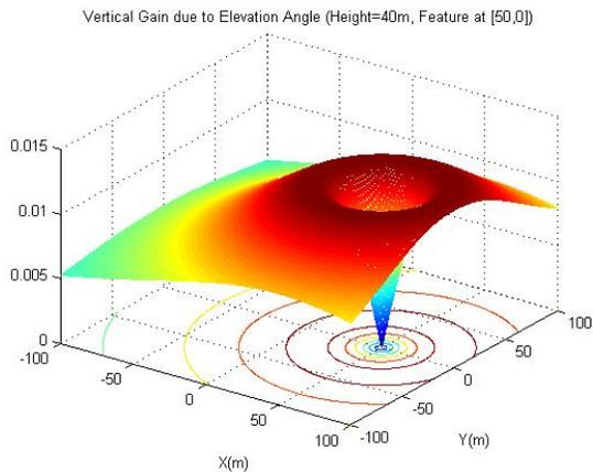
Figure 6: The vertical information gain from an elevation angle. A ground feature is simulated at  $[\pm 50, 0]m$ . It can be seen that the maximum gain can be achieved with a  $\pm 45^\circ$  elevation condition which corresponds to the top of crater.
