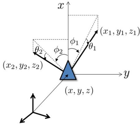
Figure 5: The sensing geometry of bearing/elevation observation from two landmarks used for analysis.
