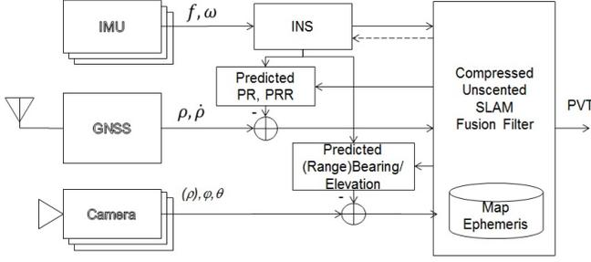
Figure 1: The system architecture for tightly-coupled GPS and inertial SLAM.
