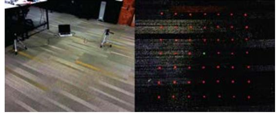
Fig. 9. Reprojection test setup (left). Reprojected grid of X and Y ranging from -300 to 300mm (right).
