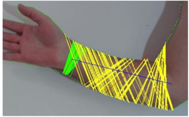
Figure 5: Green dots show outlining vector of points, green line shows possible wrist position, yellow lines show possible elbow location, red lines show wrist and elbow average location and the blue line shows the arm segment represented as a line between two points
