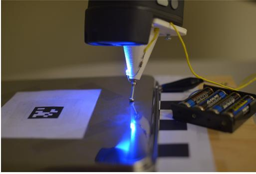
Figure 1: Touch probe equipped to the end-effector of a Baxter Research Robot
