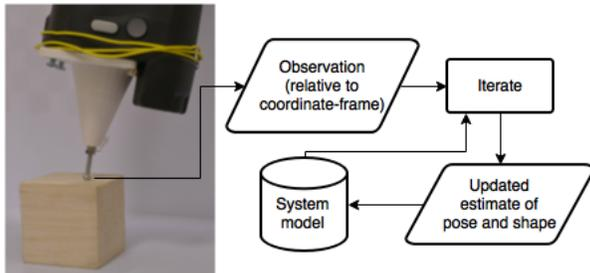
Figure 3: High-level flow-diagram showing a single observation and iteration of the filter
