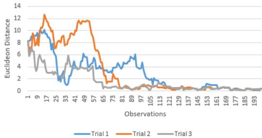
Figure 5: Graph showing the Euclidean distance between the center point of the estimate and the real object in three trials.
