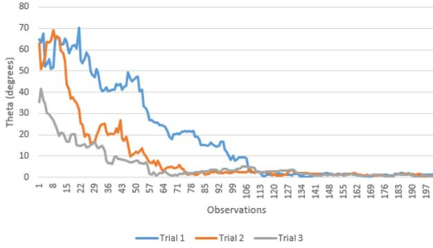
Figure 4: Graph showing the difference in rotation between the estimate and the real object in three trials.
