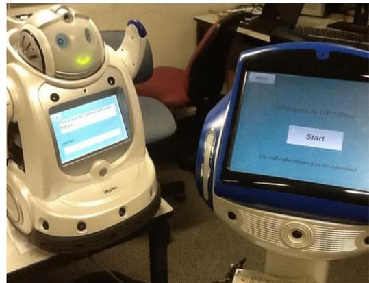
Fig. 1. Multi-robot systems with the UoA robotic software framework. The left robot is a receptionist robot to direct patients to the required healthcare services. The right robot is an assistant robot help patients to measure vital signs data, such as blood pressure, blood oxygen saturation and pulse rates.
