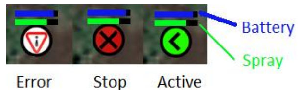
Figure 4. this figure show the three different states the robot can be in along with the battery and spray levels of each robot. The arrow shows the robot's current heading.
