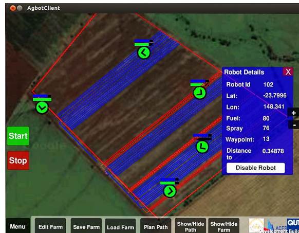
Figure 9. This screenshot shows the user interface during field trails each green circle represents an active robot. Each bar above the robot shows the battery (blue) and spray (green) levels. Completed paths are shown in red and future paths in blue. The 6 th robot in this scene has been switched off and therefore doesn't appear on the interface. The blue panel shows detailed information about robot id 102.
