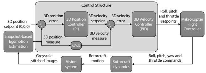
Figure 4: Onboard control structure used to control the rotorcraft’s velocity to attain the 3D position setpoint corresponding to the location of the next snapshot.
