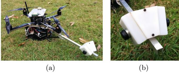
Figure 3: The rotorcraft platform used during the closed-loop experiments (a), and a close-up of the biologically-inspired vision system (b).
