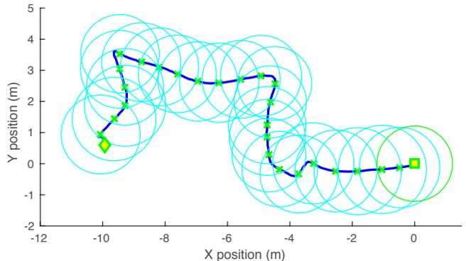
Figure 1: Route learning during a closed-loop flight test: a succession of snapshots are taken along the journey from a home position (square) to a goal location (diamond), as indicated by ground truth data. The snapshot waypoint locations are marked by green crosses and the overlapping catchment areas are shown in cyan.
