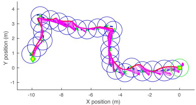
Figure 2: Long-range homing during a closed-loop flight test: the followed path back to the home location is shown in red and consists in reaching the vicinity (indicated by blue circles) of each route waypoint memorised during the outward journey (dashed blue line) to the goal location. Home and goal positions are marked by a square and a diamond, respectively. Home vectors to each route waypoint are shown in magenta.
