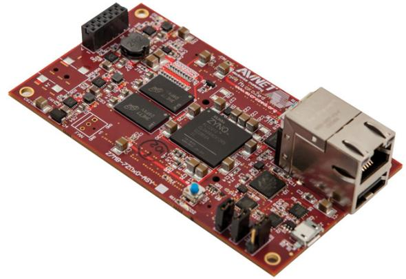
Figure 3: MicroZed Board<sup>3</sup>
