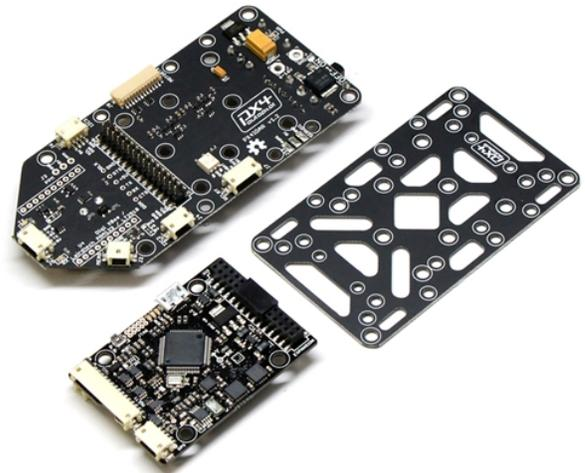
Figure 1: PX4 Autopilot Board<sup>1</sup>
