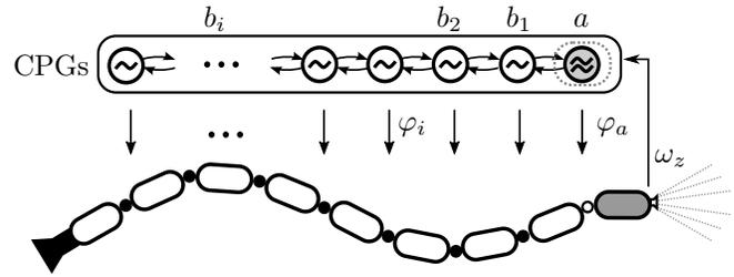
Figure 4: CPGs structure for the direction stabilisation
