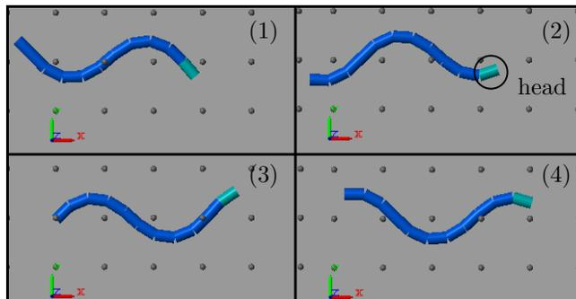
Figure 1: Locomotion of the snake robot without head stabilisation
