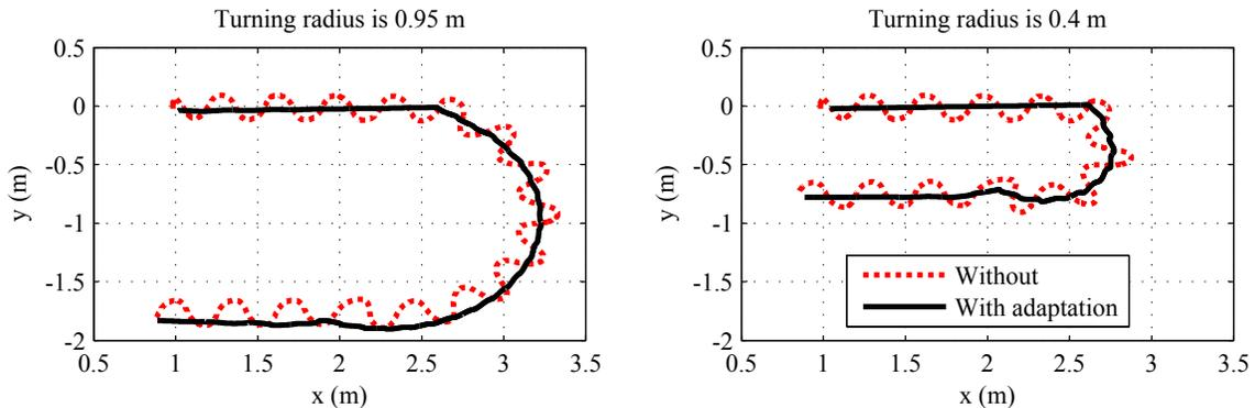
Figure 9: The path followed by the head link during turning motions
