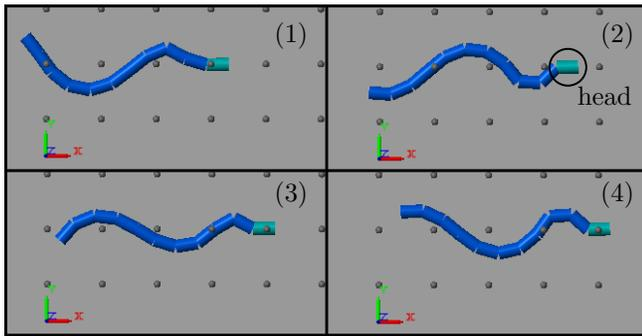
Figure 10: Locomotion of the snake robot with head stabilisation
