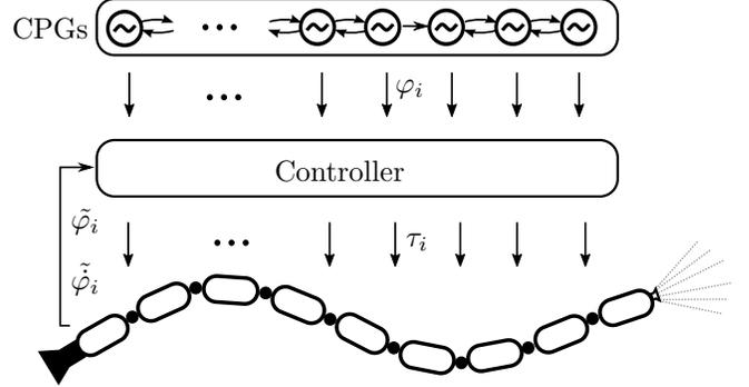
Figure 2: Architecture of the control system.
