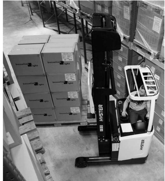
Figure 1: R1.4 Hyster Reach Truck, an example of a common FLV.
