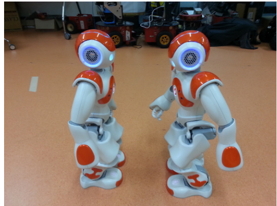
Figure 1: A pair of humanoid NAO robots communicating by encoding messages into sequences of DTMF tones. These tones can then be transmitted between robots as audio.
