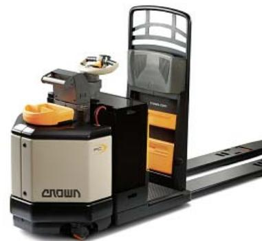
Fig. 1. Pallet Carrier, which is a platform of our forklift teleoperation system.
