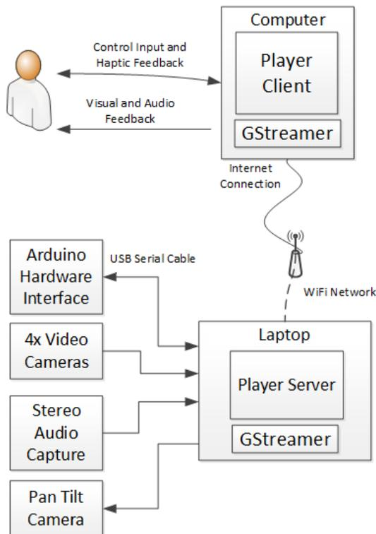
Fig. 2. System architecture of forklift teleoperation system, which consists of a laptop, an Arduino microcontroller, four cameras, a PS3 controller.
