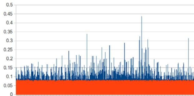
Fig. 7. Control system average round trip time latency. Localhost shown in orange, across-Auckland shown in blue.
