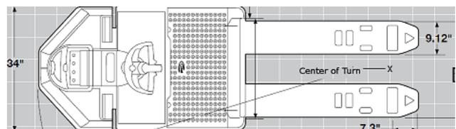
Fig. 3. Illustration of the Pallet Carrier layout.
