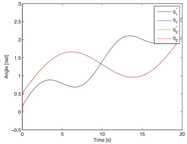
Figure 6: Link angles and its references (controller 2).
