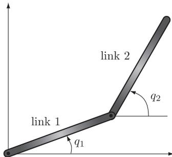
Figure 1: Two-link robotic manipulator
