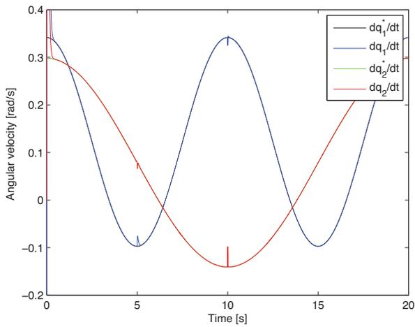
Figure 4: Link velocities and its references (controller 1).
