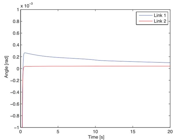
Figure 7: Angle errors  $\tilde{q} = q - q^*$  (controller 2).
