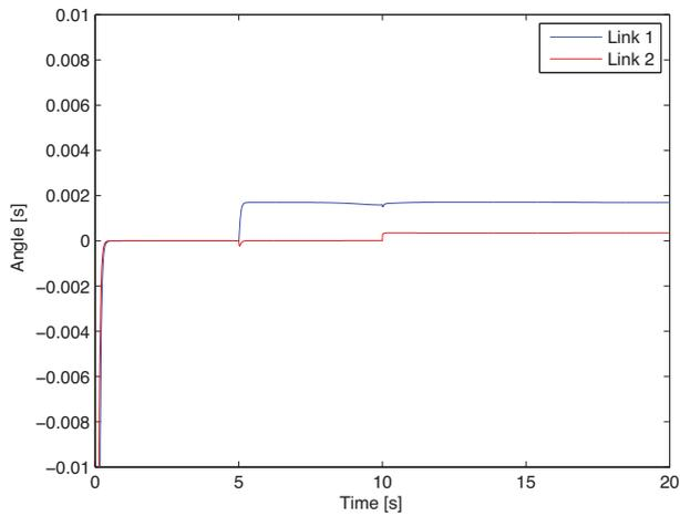
Figure 3: Angle errors  $\tilde{q} = q - q^*$  (controller 1).
