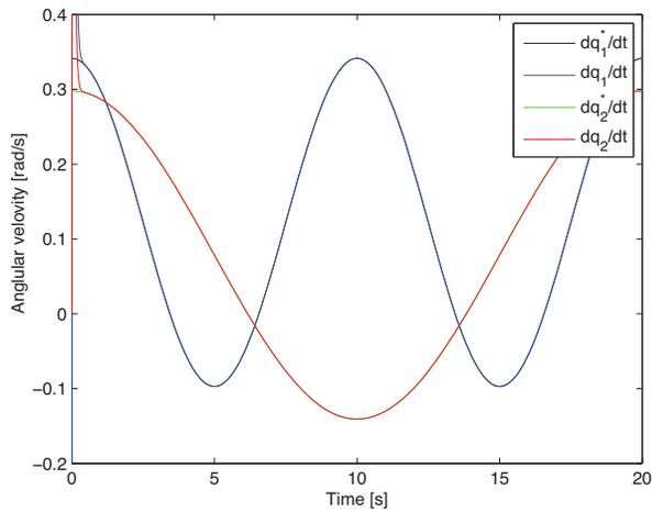
Figure 8: Link velocities and its references (controller 2).
