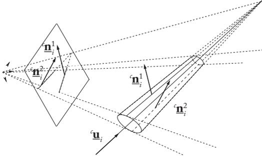
Figure 2: Projection of a cylinder in the image
