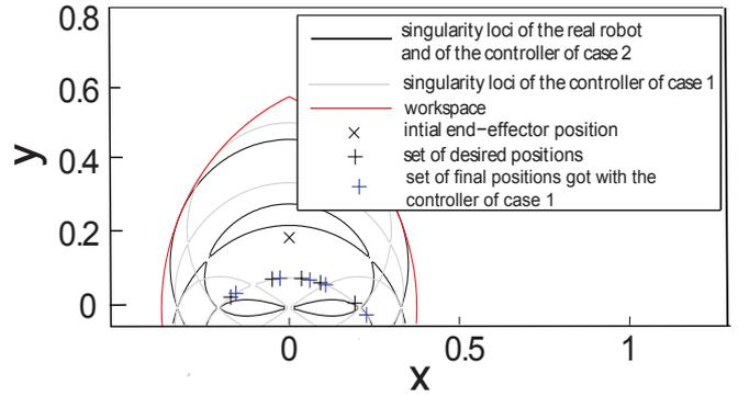
Figure 8: Singularity loci of a five-bar mechanism and its corresponding hidden robot for the following set of parameters:  $l_{1i} = 0.3$  m,  $l_{2i} = 0.35$  m,  $l_{OA_i} = 0.275$  m.
