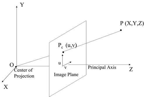
Figure 9: A pinhole camera model
