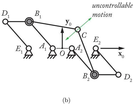
Figure 7: Examples of Type 2 singularity for a five-bar mechanism (a) and its corresponding hidden robot (b)
