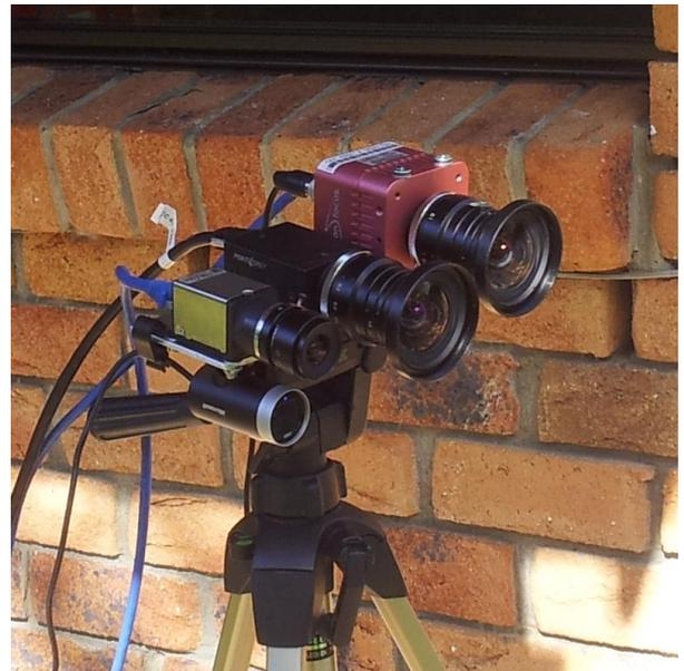
Figure 1: The dataset acquisition platform. The cameras are, top row, left to right: iDS UI-5240-CP, Point Grey GS3-U3-23S6C-C, Photonfocus MV1-D1312IE-40-G2. Bottom: Microsoft Lifecam Cinema HD
