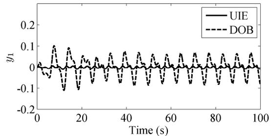
Figure 7: Closed-loop system outputs under disturbances
