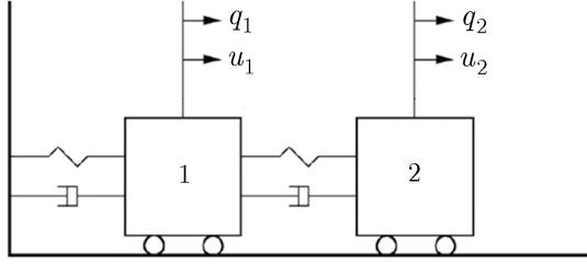
Figure 1: A mass-spring-damper system of two degrees of freedom with two control inputs (image adapted from [Shahrz, 2009])
