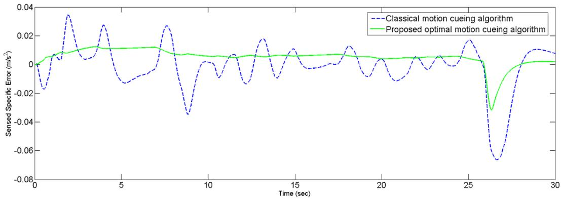
Figure 6. Longitudinal sensed specific force error comparison of proposed optimal and classical motion cueing algorithm
