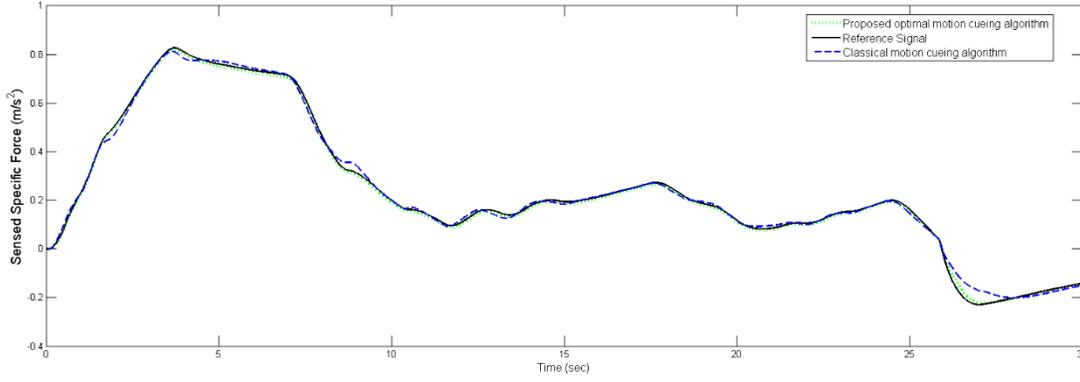
Figure 5. Longitudinal sensed specific force of reference, proposed optimal and classical motion cueing algorithm
