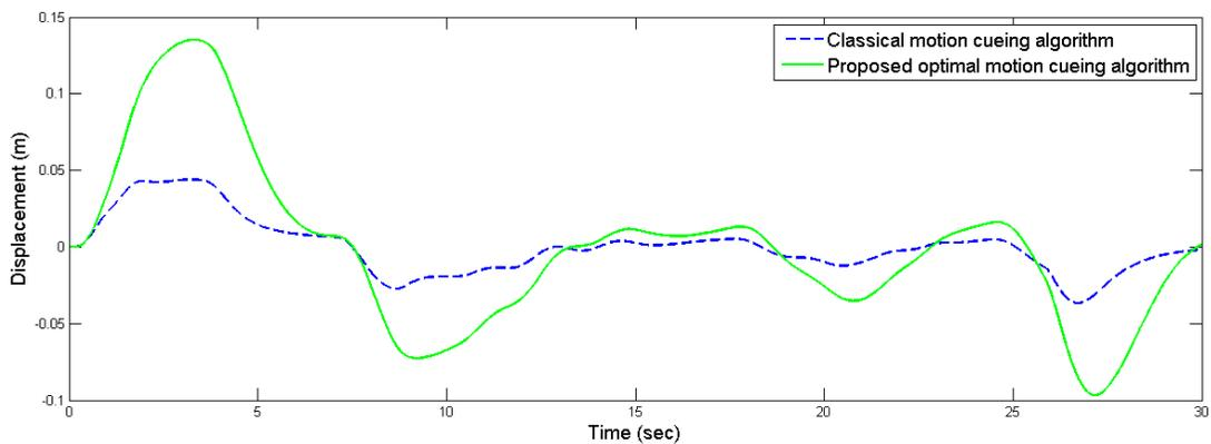
Figure 7. Translational workspace displacement comparison of proposed optimal and classical motion cueing algorithm
