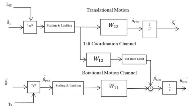
Figure 2. Optimal Algorithm block diagram for Longitudinal Mode.
