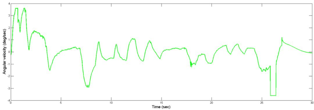
Figure 8. Optimal motion cueing algorithm angular velocity
