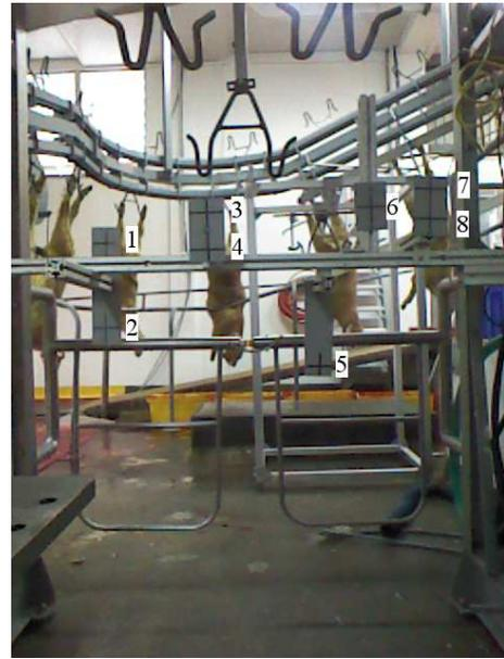
Figure 5: Calibration rig used to calibrate the vision coordinate system with the robotic coordinate system.
