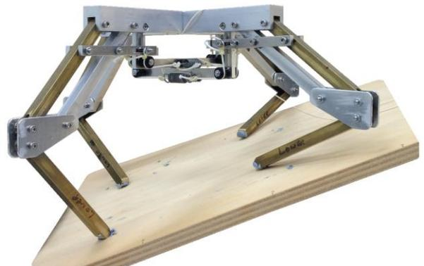
Figure 12 - Prototype Landing Gear (20 Degree Incline)
