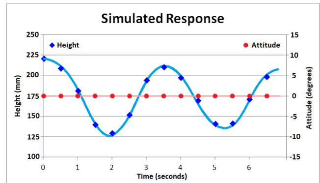
Figure 11 - Results of a simulation of the landing gear. The landing surface comprises one 25mm block and a second 37.5mm block placed on a horizontal plane resulting in tilts of 7.1° and 10.6° along the X and Y axes respectively.
