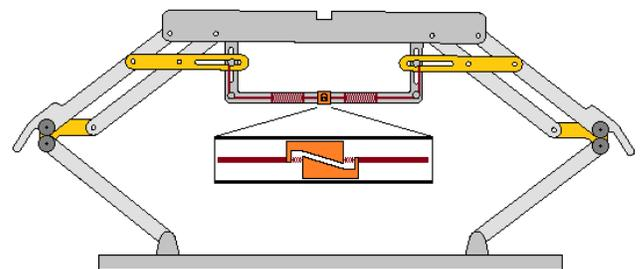
Figure 5 - Mechanical Linkage (Coupled Locking Mechanism)
