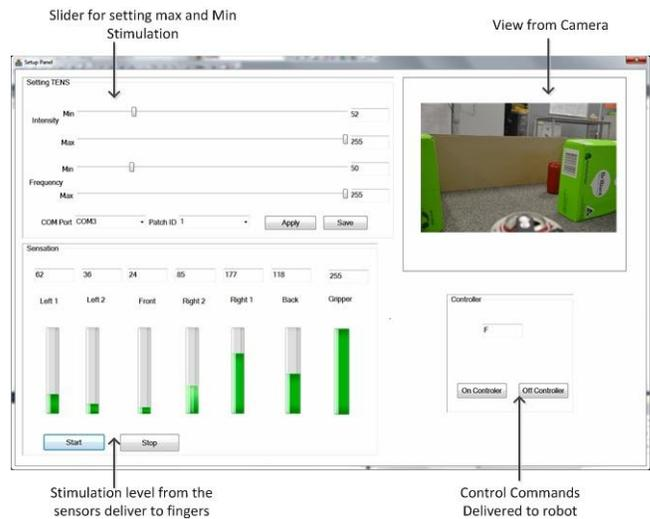
Figure 5. Electro-tactile feedback settings window.
