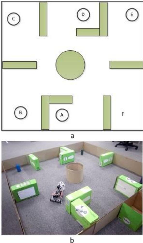
Figure 13. Obstacle avoidance obstacles experiment setup
