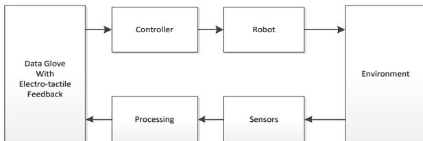
Figure 3. Block diagram of electro-tactile tele-operation system
