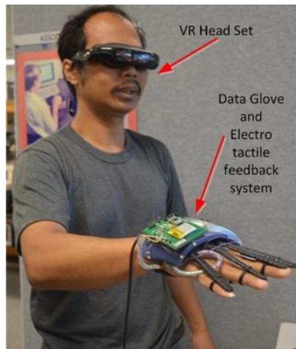
Figure 2. User with data glove and the feedback system
