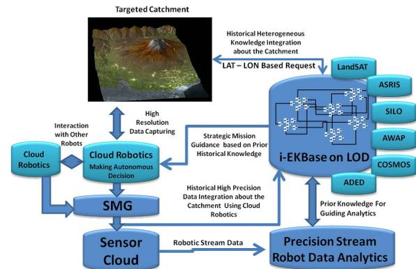
Figure 4: Architectural integration and workflow between *i-EKbase* system and Cloud Robotics via the *SensorCloud*.
