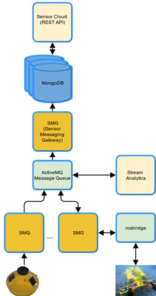
Figure 1: Scalability and the SensorCloud Robot
