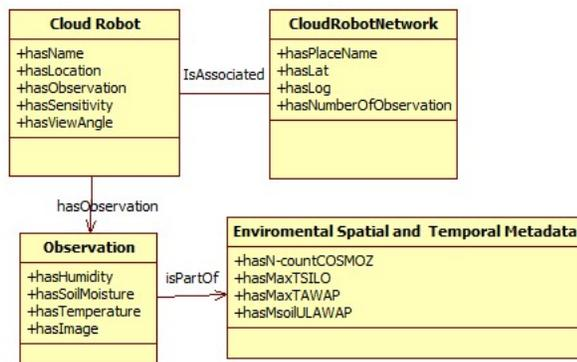
Figure 5: An example of the Robotic RDF in development.
