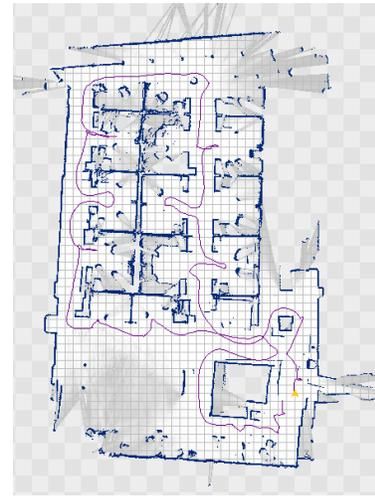
Figure 6: POG-MBICP with all laser points.
