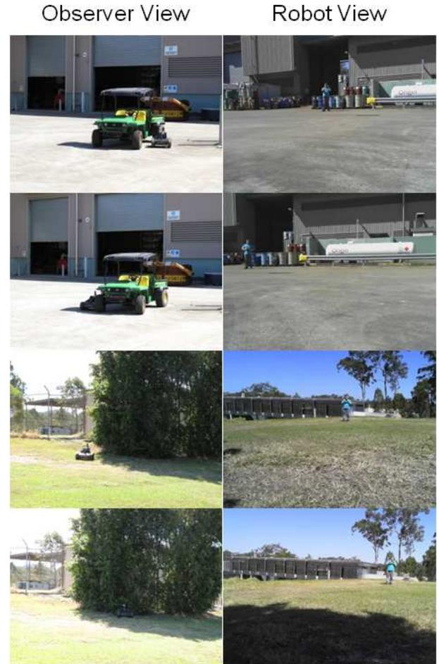
Figure 1: Four scenarios illustrating the increase covertness of the tracking robot when placing itself within a shadow compared to a non-shadow for the same vantage point/obstacle. In the top four images, the robot hides around a stationary vehicle. In the lower four images, it hides around a tree. The left images show the target's view when looking at the robot, with the right images showing the corresponding robot's view of the target.
