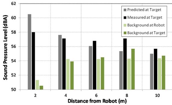
Figure 6: Measured and predicted sound pressure levels at the target from the robot moving linearly at set distances from the target. Also shown is the background SPL estimate measured at the robot and target.
