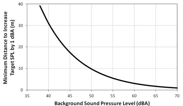
Figure 2: Example showing the minimum distance at which a robot with a 64 dBA acoustic signature must be from an observer to not increase the sound pressure level by 1 dBA with varying background noise levels ranging from still night to light industrial site conditions.
