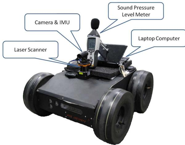
Figure 3: The robot used in the experimental campaign showing the sound pressure level meter, Hokuyo laser scanner, IMU, camera and computing hardware.
