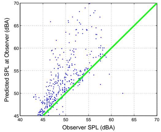
Figure 7: The robot predicted sound pressure level contribution at the target compared to the measured sound pressure level at the target for varying speed and distances. Above the green line is a conservative prediction.
