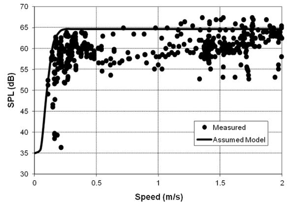
Figure 5: Variability of estimated robot SPL at 1m with robot speed, taken from day and night time experiments. The black line shows the assumed acoustic SPL model adopted for low-speed ( $< 1 \text{ ms}^{-1}$ ) experiments campaign.
