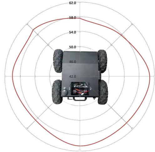
Figure 4: Measured SPL at 1m around the robot platform with motors running (no ground contact).
