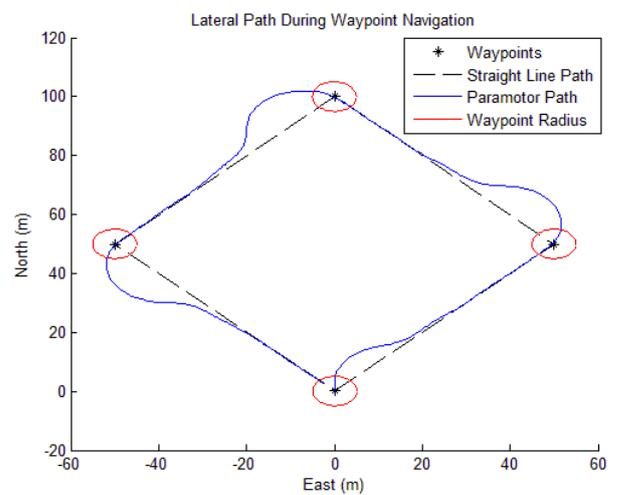
Figure 11 Simulated lateral path during waypoint navigation
