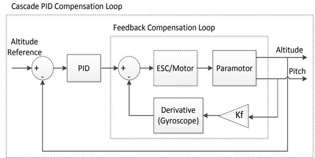
Figure 6 Altitude Hold Control Architecture
