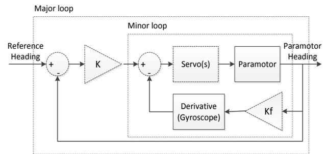
Figure 4 Lateral Control Architecture
