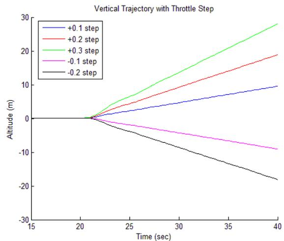
Figure 7 Vertical trajectory at different throttle settings
