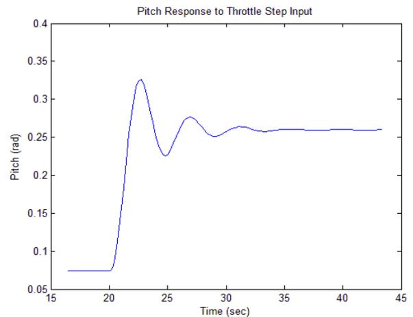
Figure 8 Pitch response of 6DOF model to throttle step input
