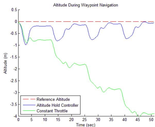
Figure 12 Simulated altitude during navigation
