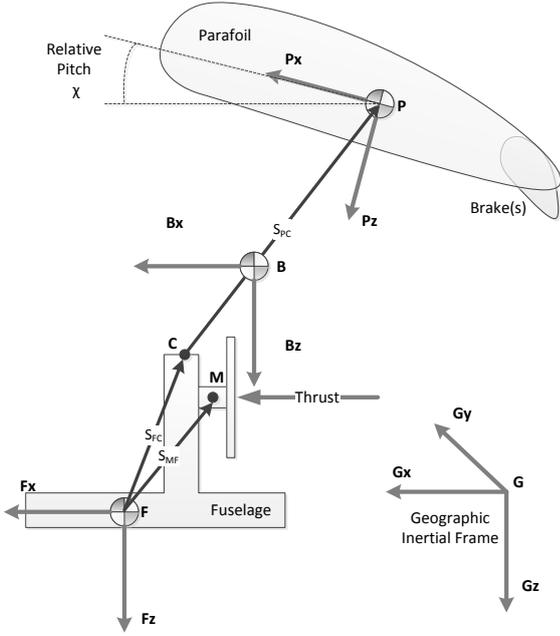
Figure 2 Paramotor Coordinate System
