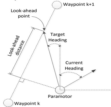
Figure 10 Guidance logic schematic
