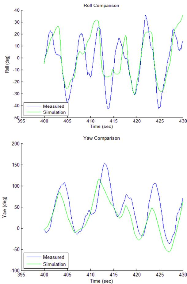
Figure 3 Comparison of Lateral Model and Flight Data
