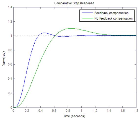
Figure 5 Step response of lateral controller with and without feedback compensation
