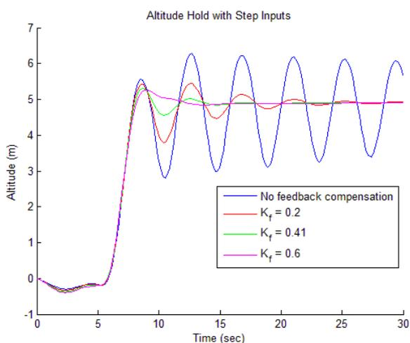
Figure 9 Altitude hold performance on 6DOF model
