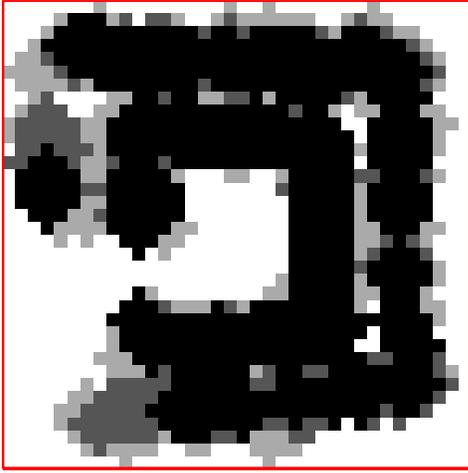
Figure 6: Dilating the entire cost map from Figure 5b by the maximum expected deformation in the map greatly overestimates the cost of traversal. The dark areas of high cost indicate the traversing the “corridors” is impossible.
