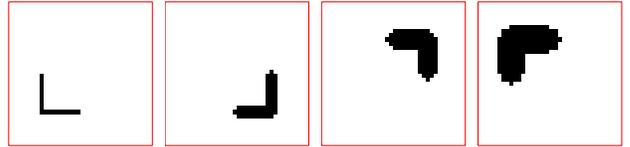
(g) Undilated section of cost map. (h) Section of cost dilated by 1 cell. (i) Section dilated by 2 cells. (j) Section dilated by 3 cells.
