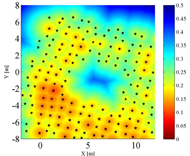
Figure 1: Maximum expected deformation of the belief state during SLAM based on sample point spacing and deformation metric values at neighbouring sample points. Sample points are shown as black stars. Higher values indicate higher expected deformation.
