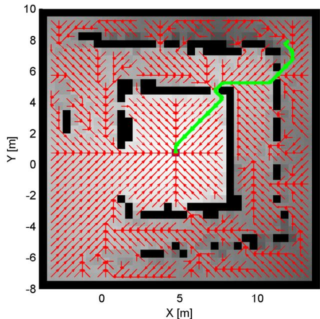
Figure 3: Global optimal policy, shown by red arrows, to reach destination at centre for the cost map shown in Figure 2b. A sample path is overlaid in green. Note in particular that the policy is optimal given the cost map and the action set. The cell colour indicates the total traversal cost to reach the destination, the summation of cell and transition costs.
