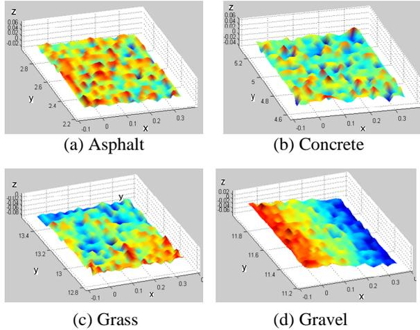
Fig. 4 Three dimensional surface data of four different road types.
