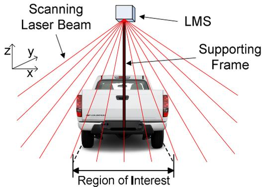
Fig. 1 The geometric arrangement of the LMS
