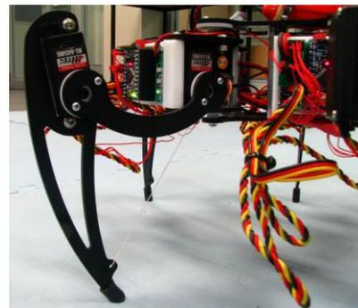
Fig. 4. Experimental Robot with Tied Leg.
