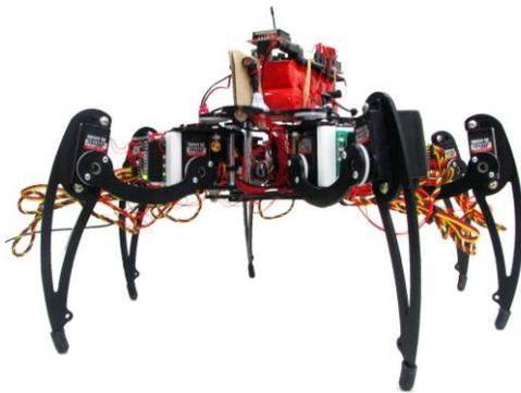
Fig. 2. Experimental Hexapod Robot.
