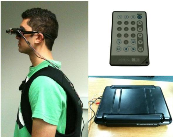
**Figure 1: Mobile simulator system (left), Infra-red remote control (top right), Hard casing for processing hardware (bottom right).**
