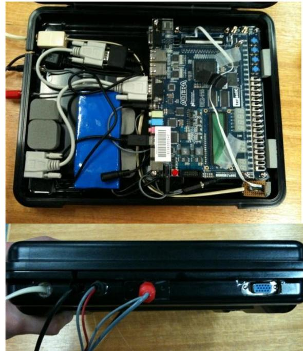
**Figure 2: Component layout within casing (top), external port connections for camera, displays and IR receiver (bottom).**
