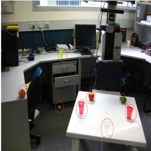
Figure 5: A snapshot of experiment setup. The potential targets are marked by red circles. They are placed at various locations, at different height and distance levels. Some of the objects are not shown in this picture due to the view of the camera.
