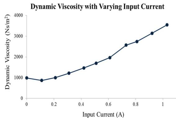
Figure 12. Viscosity dependence on current, for the compliant damper.
