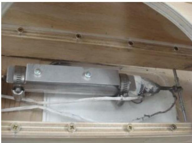
Figure 6. MR compliant damper located in the base of the system.
