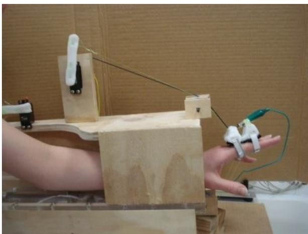
Figure 5. Test system showing the experimenter's fingers being lifted.
