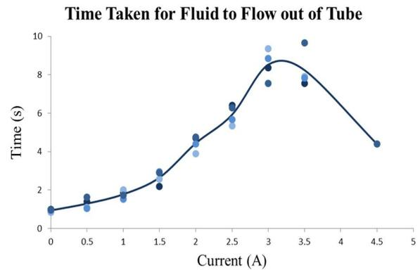
Figure 9. Heating effects influencing the viscosity of the fluid. The curve passes through the mean of each set of trials and is intended to show the general shape of the dependence.
