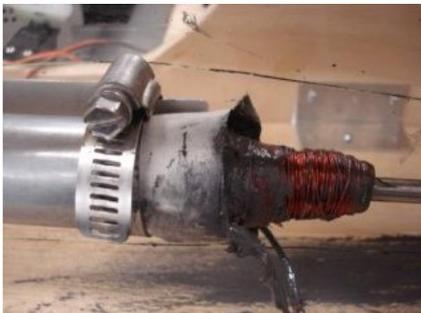
Figure 14. Coil attachment used to reduce the leaking fluid problem.
