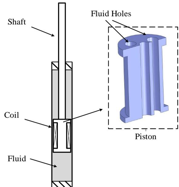
Figure 10. Cross section of the compliant damper.
