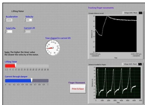
Figure 7. Screenshot of the LabView control panel showing a close-up of a current lift in progress and five previous cycles.
