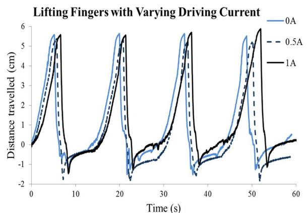
Figure 13. Time response of system when a motor was used to lift an experimenter’s fingers. Three different input damper currents are shown.
