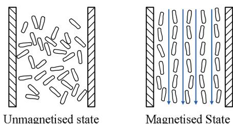
Figure 1. Effect of magnetic field on magneto-rheological fluid. The arrow indicates the direction of the magnetic field inside the fluid.
