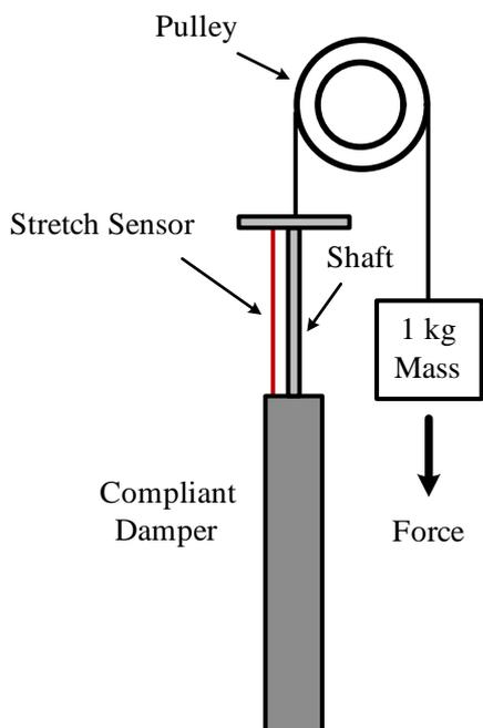
Figure 11. Schematic of the apparatus used to measure the dynamic viscosity of the fluid with varying driving currents.
