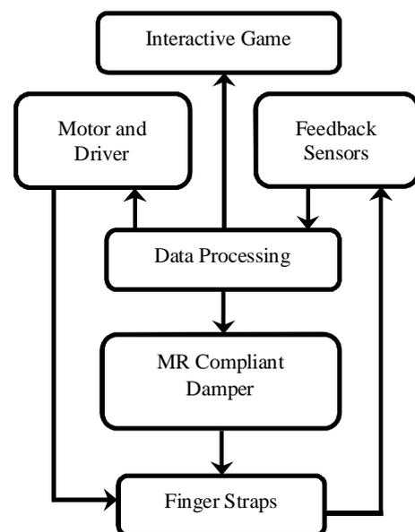
Figure 4. High level view showing the interactions of the main components of the system.
