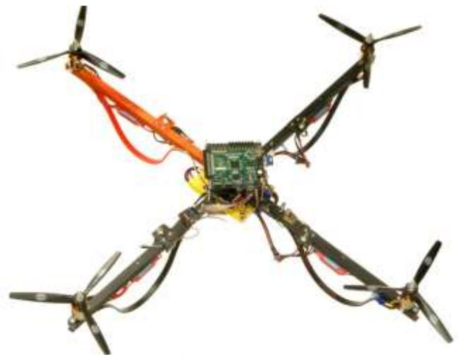
Figure 1 Quadrotor platform with FPGA board
