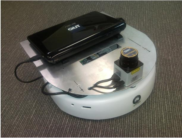
Figure 1: The robotic platform used for the experiments in this work, based on the iRobot Create hardware and ROS middleware.
