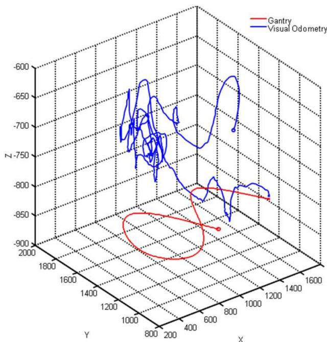
Figure 7 – Path integration performed by the sensor over a gantry trajectory. The path in the  $x$ - $y$  plane shows the sensor follows a roughly correct trajectory, but is coupled with significant  $z$ -axis position error (amplified here by a change in  $z$ -axis scale).
