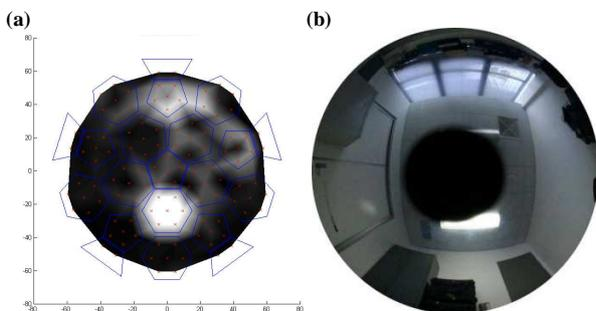
Figure 4 – Comparison between images generated by (a) the hemispherical sensor and (b) conventional omnidirectional image sensor. The occlusion in the photograph is due to the camera lens; the hemispherical sensor has a clear view of the ceiling.
