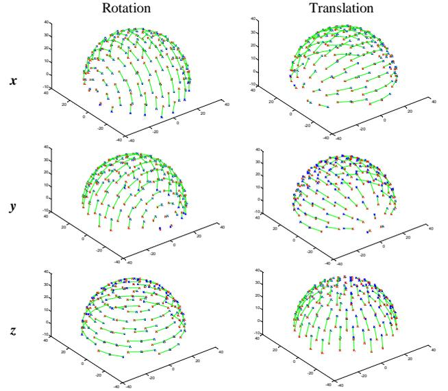
Figure 2 – Reference rotation and translation displacements for a hemispherical imaging plane. Note the similarities between rotation in  $x$  and translation in  $y$  (and conversely for  $y$  rotation and  $x$  translation) for the hemispherical case.
