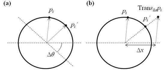
Figure 1 – The location of the point  $p_i'$  on the sphere is generated by applying either a rotation transform for image rotation as in (a), or a vector translation and remapping to the image surface for image translation as in (b).
