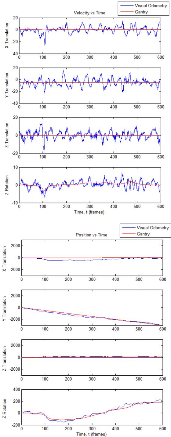
Figure 6 – Visual odometry results for (a) velocity and (b) position in decoupled camera-centred axes. Although the velocity signal is noisy, the position is correctly tracked by the sensor.
