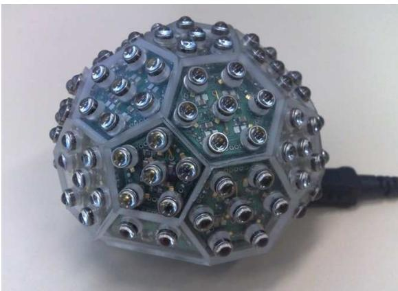
Figure 3 – Hemispherical image sensor based on the optical characteristics of the insect compound eye. The sensor consists of 116 individually lensed phototransistors arranged on a polyhedral printed circuit board, with outer alignment shell.
