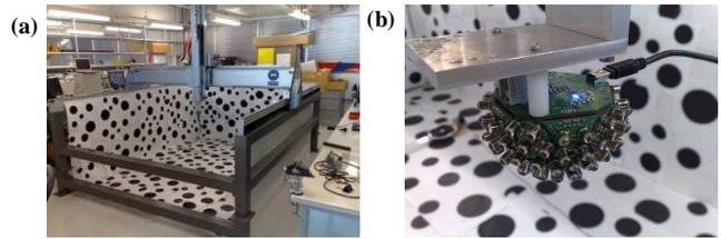
Figure 5 – Optical flow gantry. (a) shows the test pattern (with fourth wall removed) and 4DoF actuation mechanism, and (b) details the sensor attachment. The  $z$ -axes of the gantry and the sensor intersect to ensure that all motion is separable.
