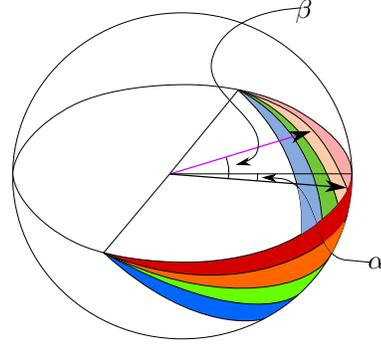
Figure 9: Construction of  $\kappa$  in the 3D case. Integration occurs across the coloured bands
