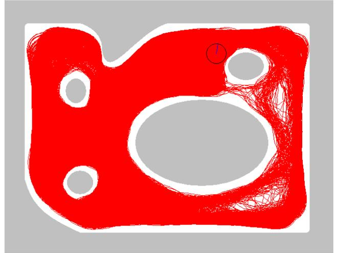
Figure 7: Noisy wall-following simulation with additional control (twelve hour simulation)
