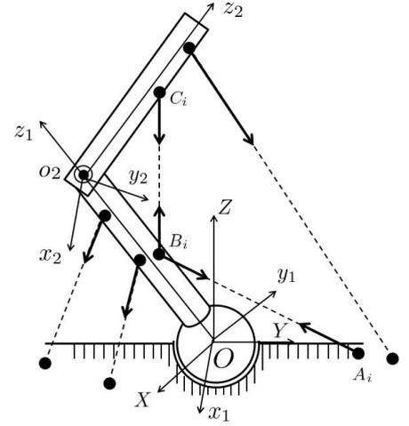
Figure 2: Model of 4-DOF Manipulator
