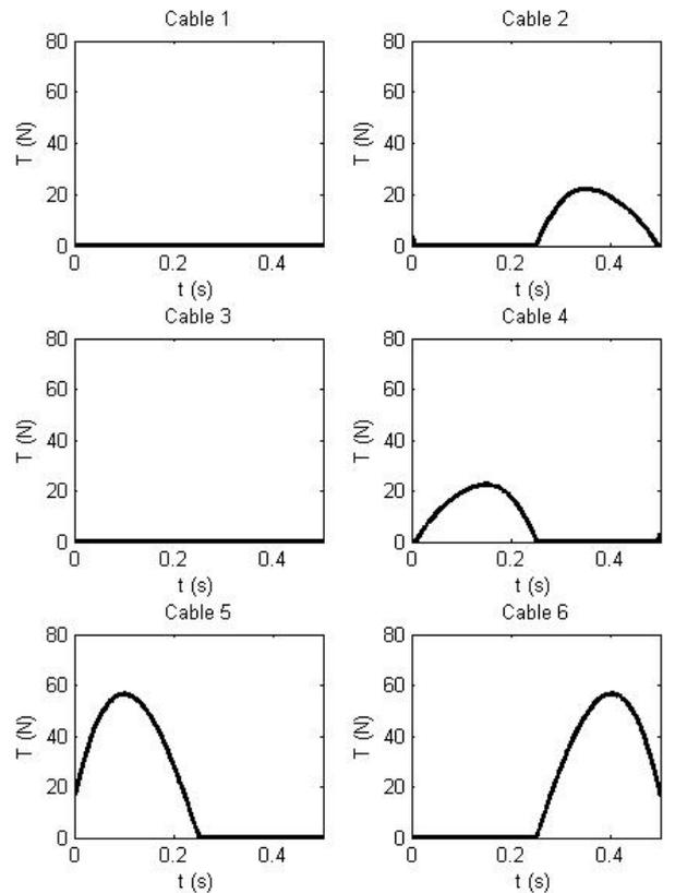
Figure 10: Inverse Dynamics for Configuration B
