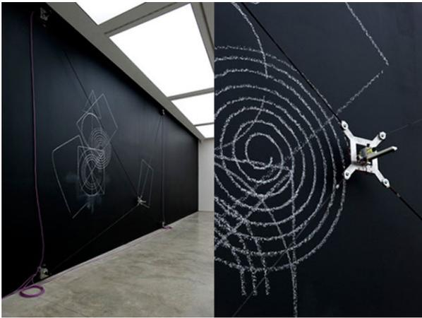
Figure 2: A chalk drawing produced by the VIKTOR painting system. The end-effector being manipulated by a four motor configuration can clearly be seen. [Lehni & Rich, 2008]
