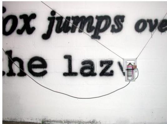
Figure 1: An output produced by the HEKTOR painting system. The spray can end-effector can clearly be seen. [Lehni & Franke, 2002]
