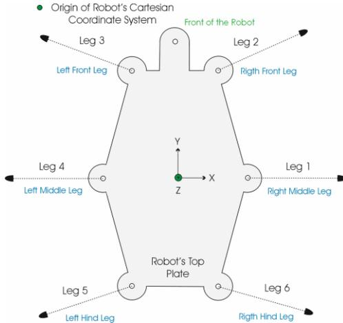
Fig. 2. Robot's Cartesian coordinate system and initial robot's leg configuration.
