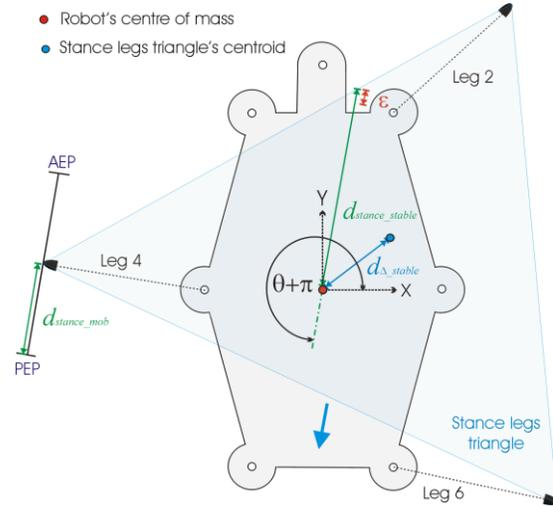
Fig. 3. Top view of a stance legs triangle including related parameters.
