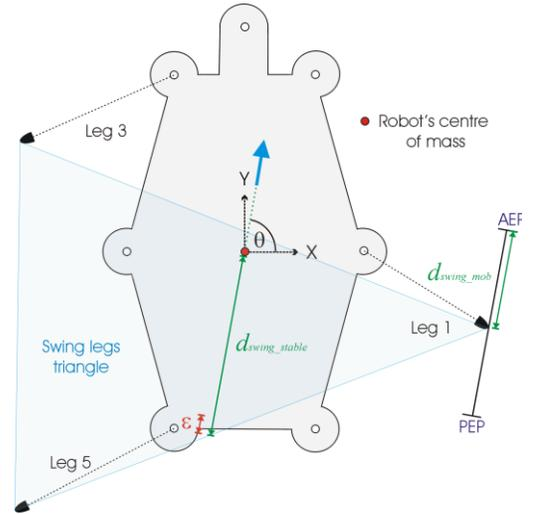
Fig. 4. Top view of a swing legs triangle including related parameters.
