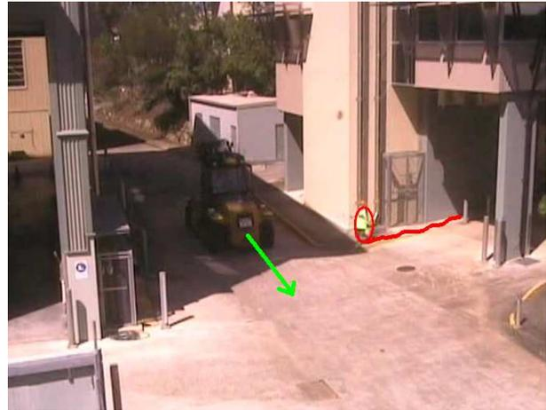
**Figure 1:** Potential collision example. The pedestrian being tracked (in red) is occluded by the building, from the truck perspective.
