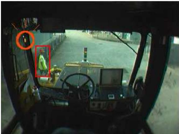
(b) Flashing light inside the cabin indicating pedestrian on the left side (shown inside the red box). While in autonomous operation, not only do the lights flash but also the vehicle slows down, according to the distance to the pedestrian and the probability of collision.
