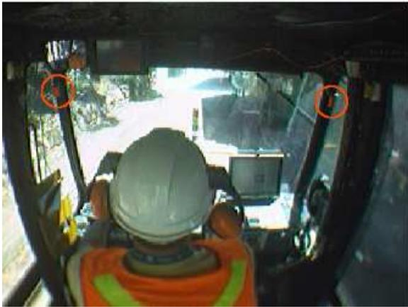
(a) Lights mounted inside the cabin, highlighted by the orange circles in this figure. During manual operation, these lights alert the driver of a potential collision route between the vehicle and a nearby pedestrian.
