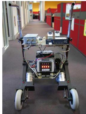
Figure 1: Rear view of the instrumented power rollator walker.
