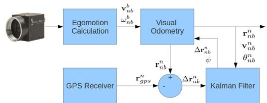
Figure 2: Proposed GPS/VO Error State Filter
