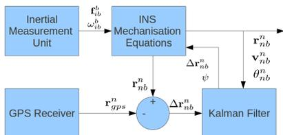
Figure 1: Classic Loosely-Coupled GPS/INS Error State Filter
