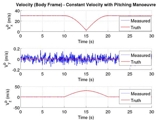
Figure 8: Scenario 2, Velocity in the b-frame. Note that although the velocity in the body frame is changing, the velocity in the navigation frame is not.
