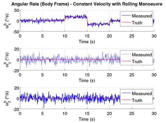
Figure 3: Scenario 1, Angular Rate Inputs with the platform performing a roll manoeuvre
