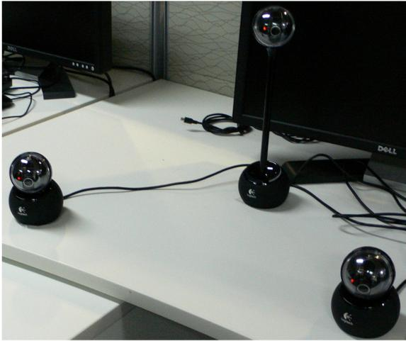
Figure 1: An example pan-tilt-zoom camera array. The cameras are steered to maintain gaze towards a common point in the workspace.
