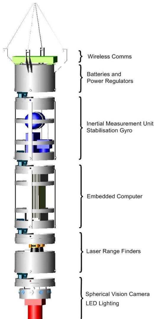
Figure 5: Exploded view of mark II pod
