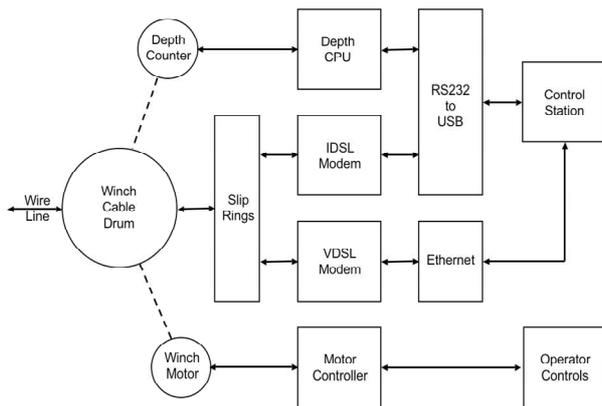
**Figure 1: Deployment and monitoring systems**
