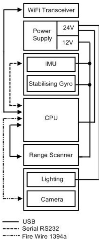
Figure 6: Data sensing system (pod)
