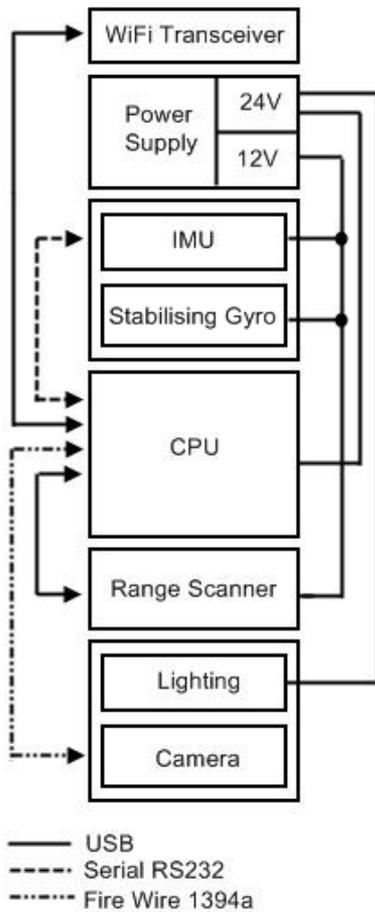
Figure 6: Data sensing system (pod)
