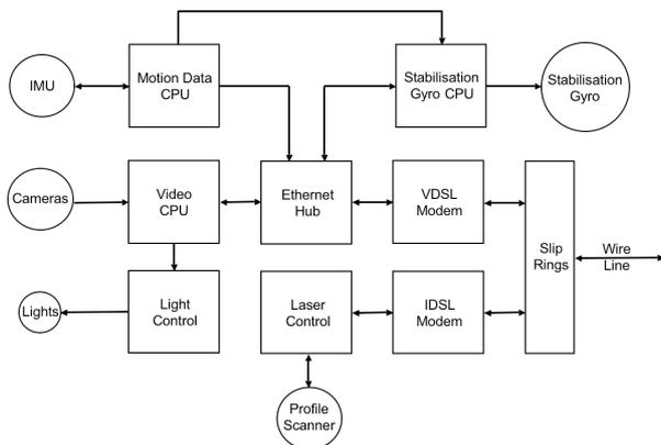
**Figure 2: Data sensing system (pod)**
