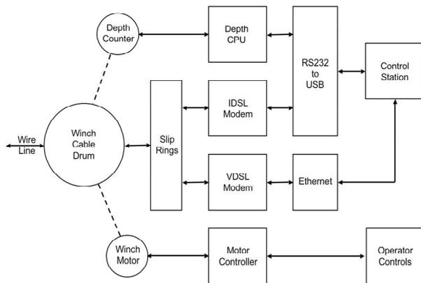
**Figure 1: Deployment and monitoring systems**
