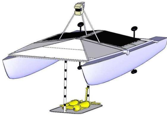
Figure 2: Conceptual diagram of AUV docking system slung underneath the CSIRO developed Nikki Autonomous Surface Vehicle.
