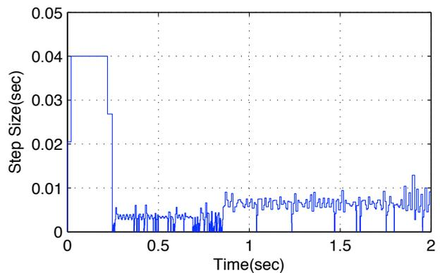
Figure 9: Rigid bar colliding with ground (normal force: Linear S-D 1 , friction force: Double state friction)
