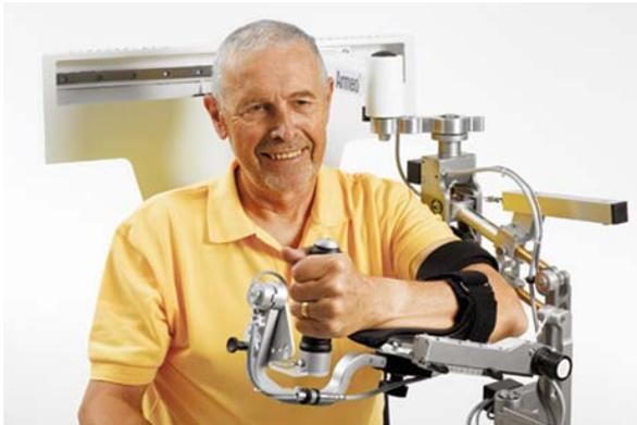
Figure 2. ARMEO – a passive exoskeleton device
