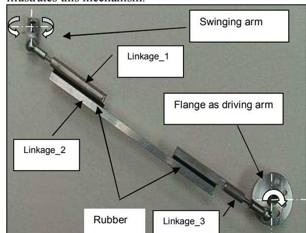
Figure 3: Four-Bar Linkage Mechanism
