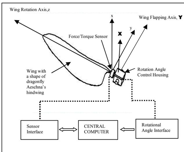
Figure 2: Top Rear View of the Device
