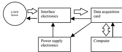
Figure 6. Schematic of the Data Acquisition System
