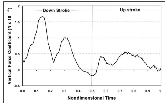
Figure 10. Experimental results for lift force coefficient
