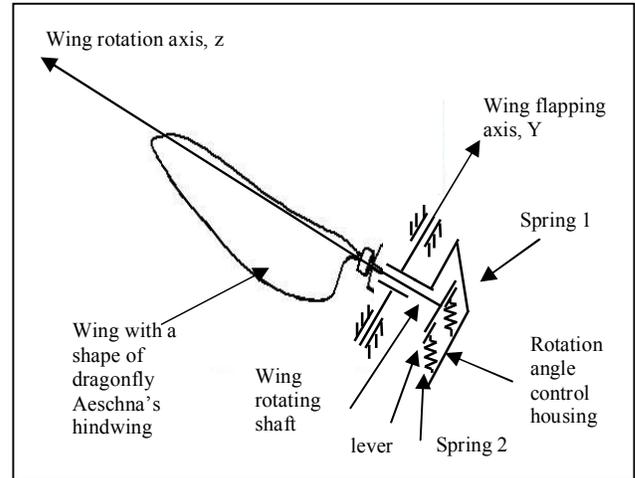
Figure 4. Wing Rotation Control Unit
