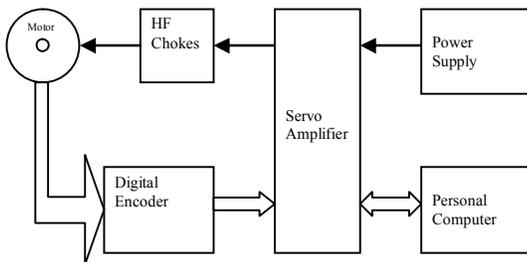
Figure 5. Schematic of Electrical System
