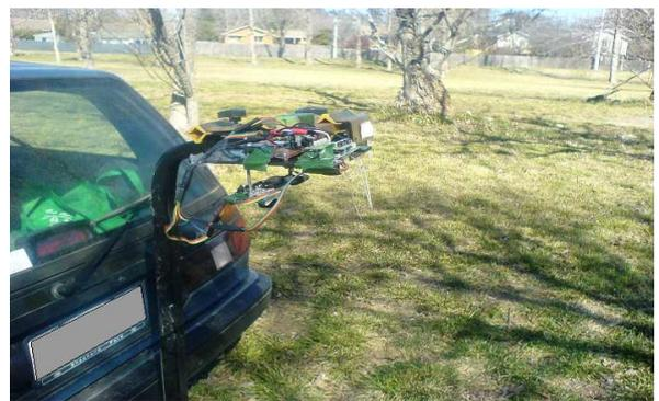
Figure 5: A differential Optic-flow system installed on a car bike rack
