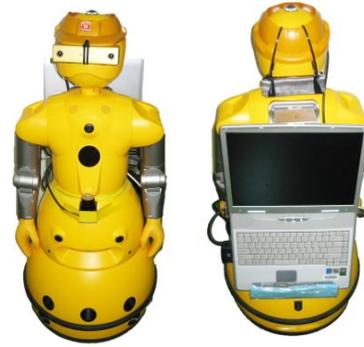
Figure 1: Wakamaru with Bumblebee camera on head, HokuyoURG laser range finder at middle and laptop on back.
